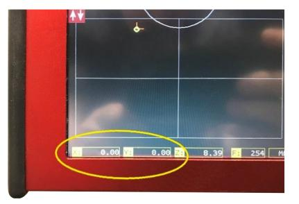
Now, manually move the robot arm and stylus to the CONE TIP at rail #3. (the cone tip at the furthest position from the face of the ArcDroid<sup>M</sup>).
